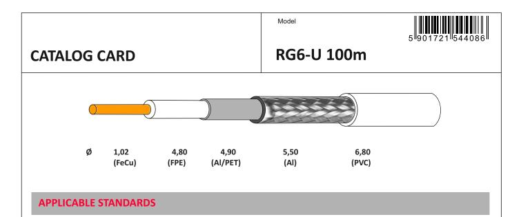
1. PN-EN 50117-2-4: 2005+A1:2008. Coaxial cables - Part 2-4: Sectional specification for cables used in cabled distribution networks - Indoor drop cables for systems operating at 5 MHz - 3 000 MHz.
